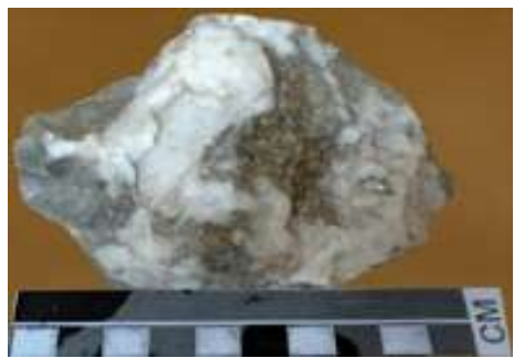
Figure: (13 a, b, c and d) Nature of gold mineralized quartz veins in research area
